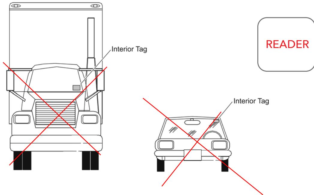
If the UHF reader antenna is installed to the right of the vehicle, optimal tag position is on the **right side** of the vehicle.
