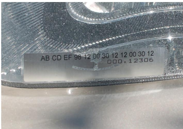
**STEP 2:** Apply protective overlay over headlight tag.
