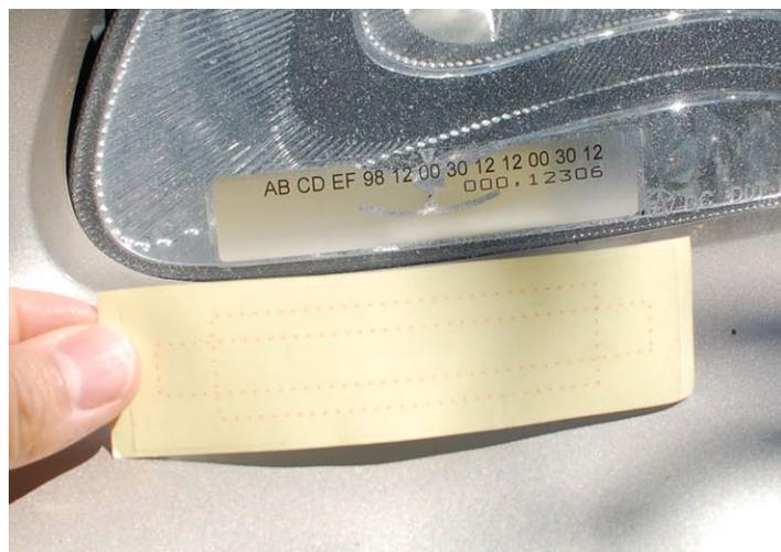
**Installed tag with protective overlay:**
